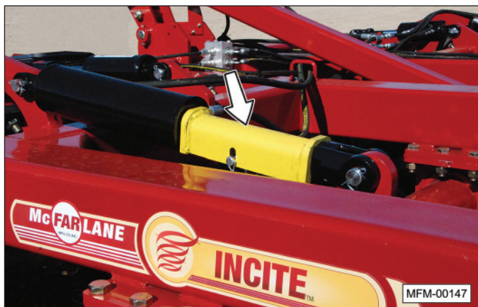
Transport lock secured over cylinder rod.
