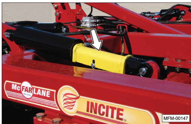
Transport lock secured over cylinder rod.
